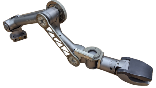
Fig. 3: Unitree Z1 Pro arm . This arm’s harmonic actuators behave substantially differently from the quasi-direct-drive motors common in small legged robots. This image also shows the reinforcements we designed to ensure that the limit on athleticism comes from actuation rather than the linkage structural integrity.
