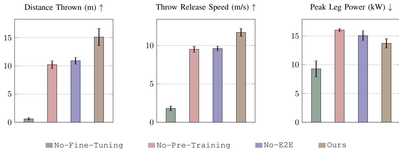
Fig. 5: End-to-end fine-tuning from a pre-trained WBC leads to the best task performance. Throwing evaluation metrics across 100 simulated throws for four policies: Our fine-tuned WBC ( Ours ) achieves the longest throw distance with lower peak leg power as compared to a throwing policy trained from scratch ( No-Pre-Training ) or a high-level policy for a frozen WBC ( No-E2E ). The WBC before finetuning ( No-Fine-Tuning ) has the lowest peak leg power but throws the ball a much shorter distance.
